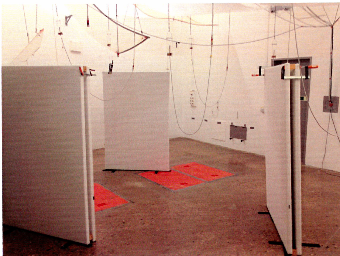
Figure 1. The figure shows the test set up, where three couples of screens were mounted toward each other with 30 mm air gap between the screens.
